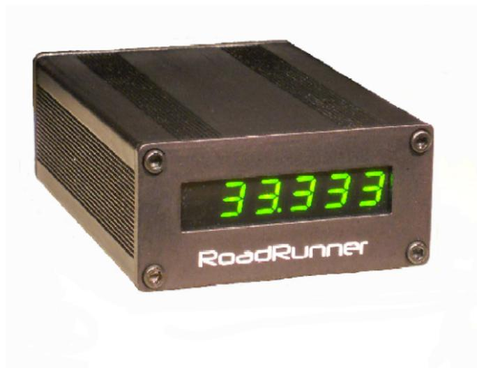
The RoadRunner is a microprocessor controlled digital tachometer used for monitoring turntable platter speed to 3 decimal places of resolution. The internal time base is a temperature compensated crystal oscillator (TCXO) accurate to 2.5 PPM ( $\pm 0.00025\%$ ) with less than 1.0 PPM aging per year.
